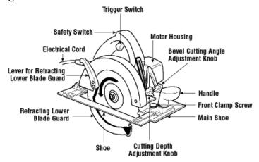
The above diagram shows the important features on most circular saw models. These components can be broken into three groups: safety features, saw adjustments, and places to grip the saw.
