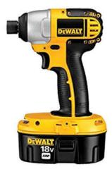
An impact driver is a driver that has more torque and power than a normal drill. They are generally helpful when screwing more difficult wood such as two 4x4s or when using large hardware such as lag bolts. Impact drivers have a "collet" that only accepts hex shaped bits. To insert the bit, pull back the collet and place the bit into the slot. Once the collet is let go of, the bit is secured.
