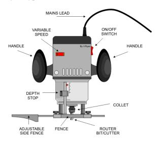
Routers are designed to be operated with two hands, one holding each handle. The tool is powered on by a single switch and the speed of the tool can be adjusted. The depth stop allows the user to set the depth of cut for the tool.
